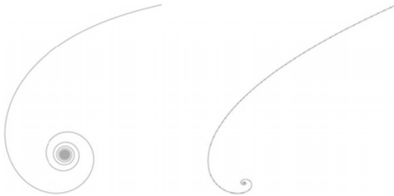
Figure 6.9 Left: A spiral path that is not smooth. Right: A smooth spiral path.
